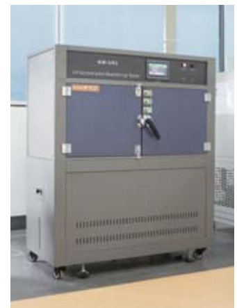
UV老化环境试验机 UV accelerated weathering tester
