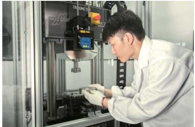
Wa Zau 材料摩擦磨损试验机(德国) Wa Zau material friction&wear tester (Germany)
