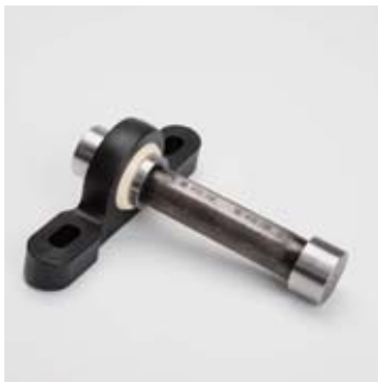
正确：采用塞规检测 Tolerance test with plug gauge
